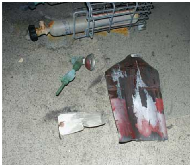
A lecture bottle of anhydrous HF ruptured at the UC-Santa Barbara. Debris shattered the heavy-duty glass of the gas cabinet before striking a wall 10 feet away.
