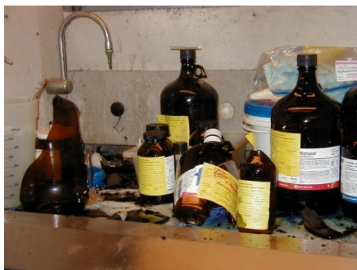
Figure 1. Nitric acid was collected in a methanol container. The reaction caused the container to burst into tiny pieces strewn throughout the lab. Several nearby containers broke. The lab was closed for two days for cleanup.
